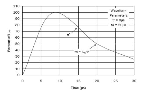
Fig.2 Pulse Waveform
