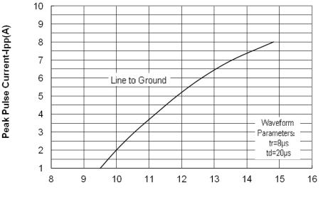
Clamping Voltage-Vc (V)
