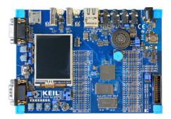
The Keil MCB1800 Evaluation Boards enable you to create and test working programs based on the NXP LPC1850 family of ARM Cortex™-M3 processor-based devices.
